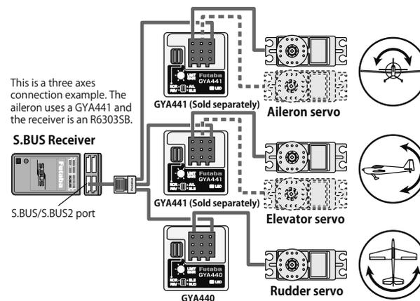
S.BUS connectivity minimizes wiring. The GYA441 and GYA441 can be connected by one 3-way hub. The aileron, elevator, and rudder servos are output from the gyro. Standards servo can also be used. When an R63035B is used the CH switching mode is set to group 7. The normal group 7 CH outputs are CH3, CH11, and CH12. CH3 is the throttle channel and CH11/CH12 are spare channels.
