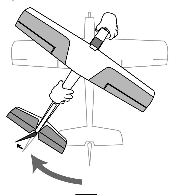
Tilt the airplane to the left on the ground and check that the ailerons
