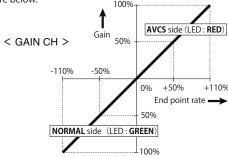
3CH (GAIN CH) is set up with reference to the manual of a transmitter. Neutral position becomes GAIN 0%. It is divided into AVCS side and NORMAL side. Check using the GYD450's LED.
