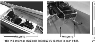
\*The main purpose of the photo demonstrates how the antenna should be placed. For actual installation the receiver must be wrapped with a sponge or placed with floating material to protect it from vibration.
