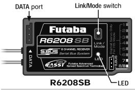
Channel outputs for conventional system (1 to 8)
