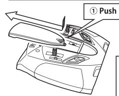
② Remove the battery cover from the transmitter by sliding it to the direction of the arrow in the figure.
