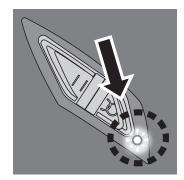
(If voltage is about **4.0v** or less, a **blink** indication of the **LED**.)
