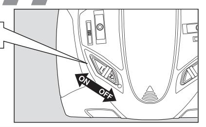
If the power switches are turned off in the opposite order the model may unexpectedly run out of control and cause a very dangerous situation.
