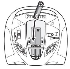
3 Prepare the new AA size batteries. Pay very close attention to the polarity markings and insert accordingly.
