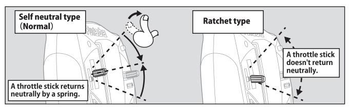
Open the transmitter front case and modify the stick section.
