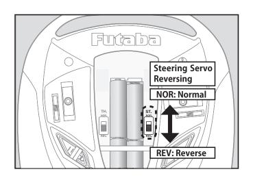
Change the direction of the steering reversing switch.
