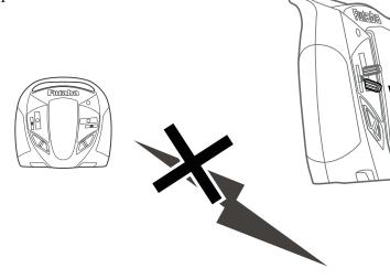
For the engine car, link the transmitter and the receiver at braking position.
