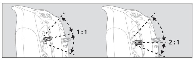
Change the neutral position only when large forward stroke of the throttle stick is need when using an FET E.S.C., etc.
