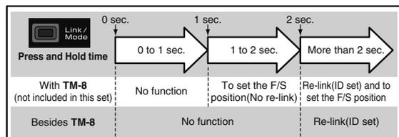
\*Refer to the instruction manual of the transmitter or module used for a description of the linking operation, F/S position setting methods and other details.
