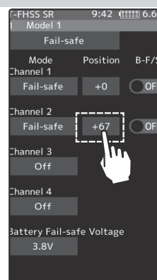
Fail-Safe position setting While holding the stick, tap the Fail-Safe position button.
