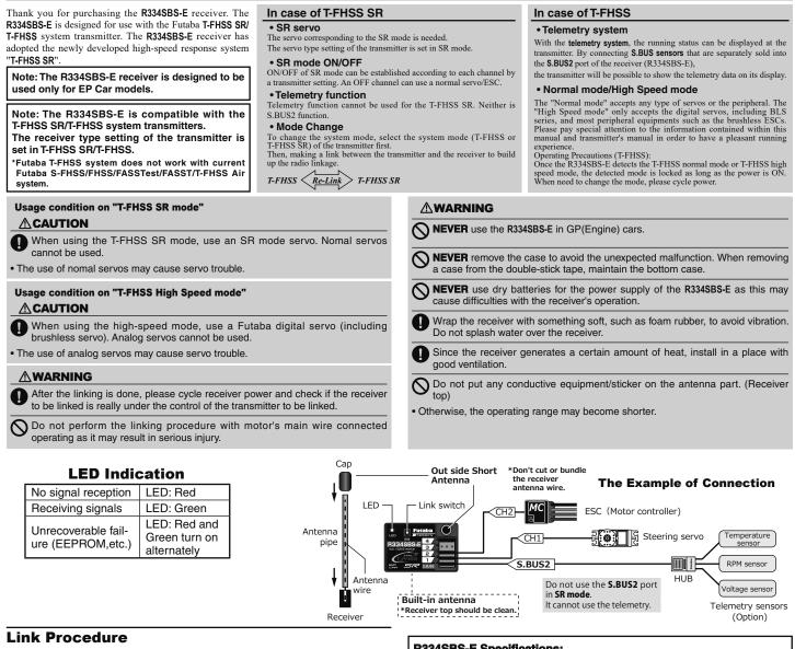
Each transmitter has an individually assigned, unique ID code. In order to start operation, the receiver must be linked with the ID code of the transmitter with which it is being paired. Once the link is made, the ID code is stored in the receiver and no further linking is necessary unless the receiver is to be used with another transmitter.
